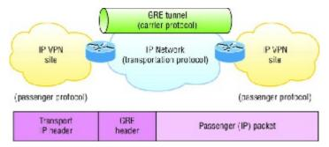
FIGURE 21.23 Generic Routing Encapsulation (GRE) tunnel structure
